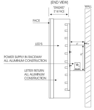
INSTALLATION: 3/8"X4' LAG BOLTS, 4 PER LETTER OR AS NEEDED (MAY REQUIRE OTHER TYPES OF FASTENERS DEPENDANT OF WALL)
